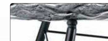
i Hinged beams at the upper side of the trestle can be adjusted individually to the shape of bowls and platters
